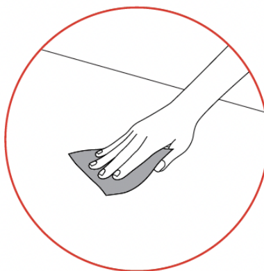
Intense clean/repair Use finest grade sand/glass paper applying only light pressure to restore surface
