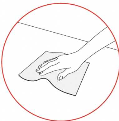
Regular cleaning Use a soft cloth or sponge and mild detergent for regular cleaning
